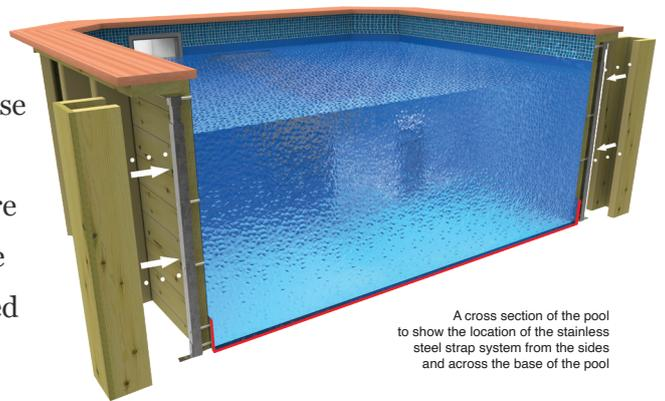
A cross section of the pool to show the location of the stainless steel strap system from the sides and across the base of the pool
